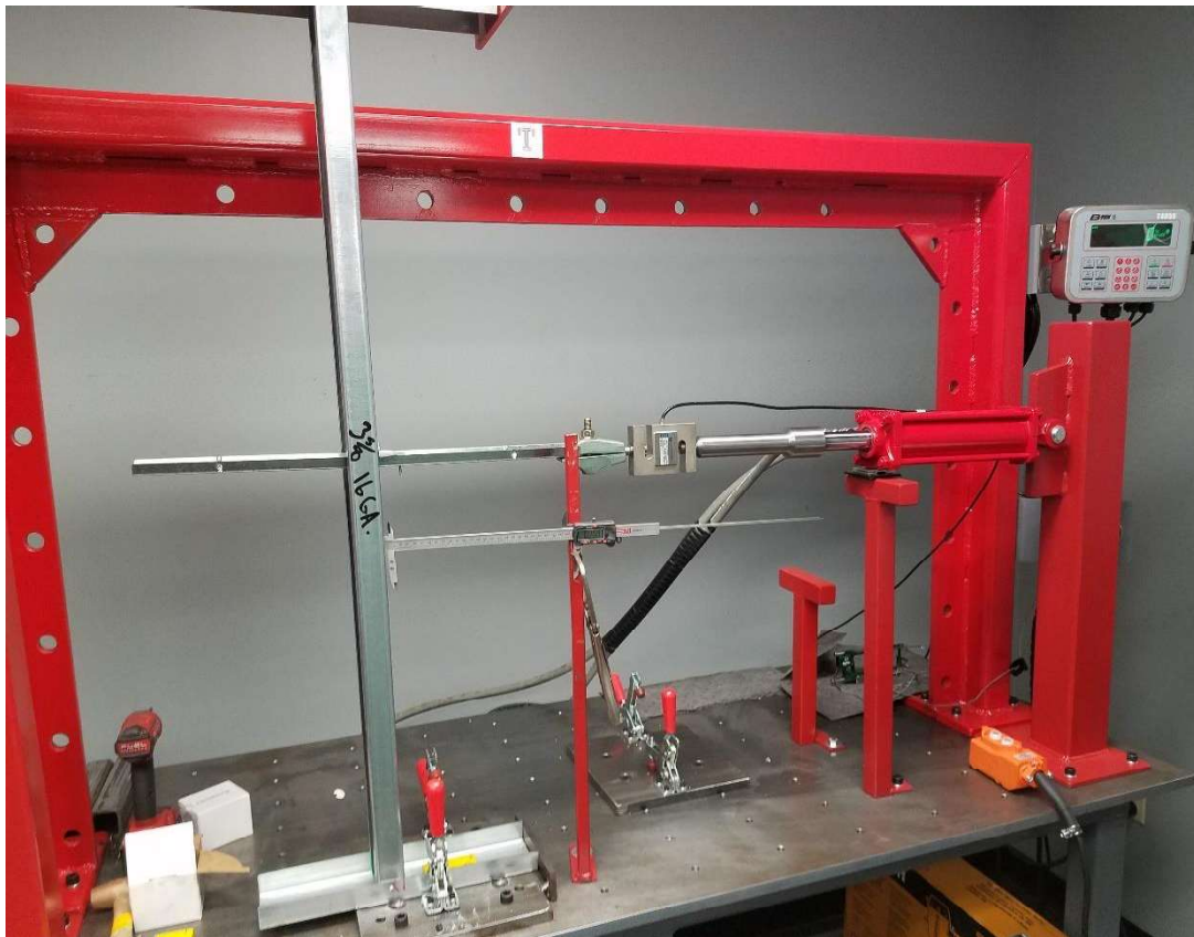
Figure 4-1: Photograph Lateral Loading Test Set-Up
