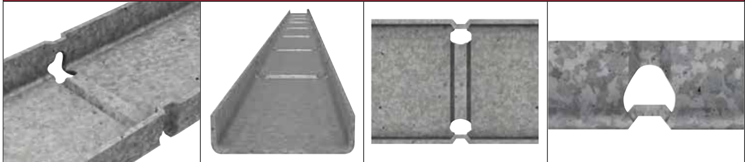
T-Brace with self nesting geometry to fit one part inside of another and secured with a screw. T-Brace locking features spaced every 4" to accommodate 12", 16" and 24" on center stud spacing.
