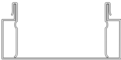
VersaDry with clip at floor without caulk
