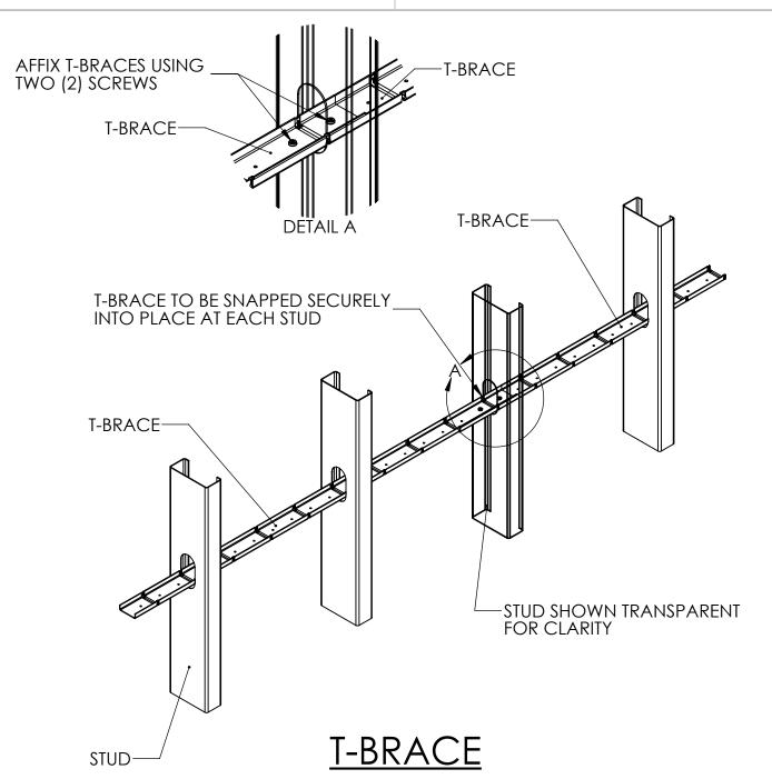
NO CLIPS OR WELDING IS REQUIRED FOR MOST NON-STRUCTURAL APPLICATIONS. HOWEVER IF ADDITIONAL BRACING IS NEEDED, CLIPS CAN BE INSTALLED AS SHOWN.
